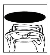
5. Remove grille and insert unit into hole.
