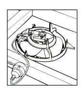
It is recommended that the three sliding clamps be checked for the correct clamping by inspection from above.
