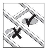
Determine position in ceiling where the Exhaust Fan is required to be installed. (Do not install within 120cm of stove or inside a shower recess).
