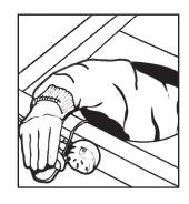
4. The Exhaust Fan is supplied with lead and 2 pin plug. Ensure that a power outlet is installed near the fan. (This outlet may be controlled by a standard switch or time delay switch.) Check power to the outlet is off. Plug the fan into this power outlet.
