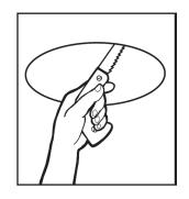
3. Use electric jig saw or small hand saw to cut out around this line. Several holes drilled at a point inside the circle provides a convenient starting point for cutting the panel out.
