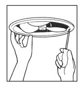
6. Tighten the screws until the sliding clamps securely grip the ceiling material (0.5 - 0.6 Nm).
